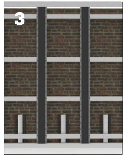
3. Connect the frames with „shadow” panels. Mount masking panels at the bottom and top.
