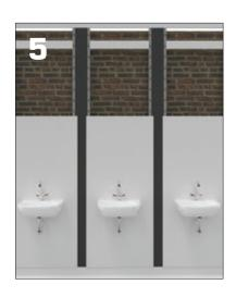
5. Secure and connect the fixtures to the cladding.
