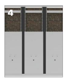
Fit the cladding panels up to the height of the utilities and fixtures. For the cladding where fixtures will be installed, cut openings for the connections/fixtures.
