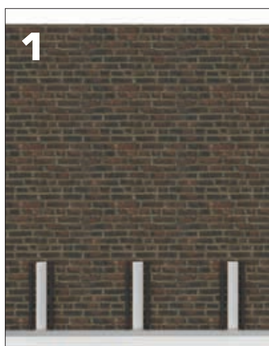
1. Level and mount the bottom profile to the floor.
