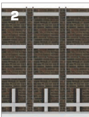
2. Place the steel frames for cladding on the profile, align, and attach them to the masonry wall.
